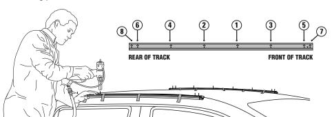
Check both tracks are secured to the vehicle as per these installation instructions. For assistance, contact your local dealer.
