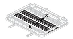
Install Restraint Clamp onto outside ridge of the chosen inner tray slat and secure to Restraint Mount with M8 Washer, M8 Spring Washer and M8 Set Screw. Use a 13 mm spanner to tighten screws to 14 Nm.
